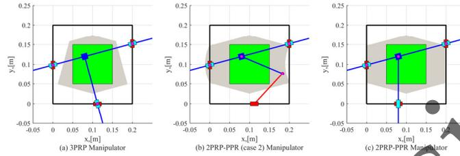
Fig. 8 Singularity-free workspace for  $[-15^\circ, +15^\circ]$  along with the accuracy test region
