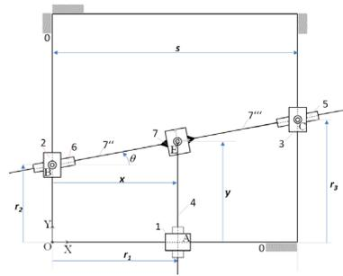
Fig. 6 Schematic arrangement of the planar 2PRP-PPR parallel manipulator
