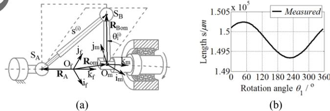
Fig. 2 Accuracy testing of an R-pair with ball bar and the measured data
