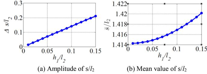
Fig. 9 The relationships between  $s/l_2$  and  $h_1/l_2$
