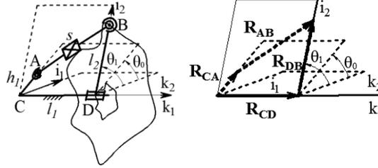
Fig. 5 The spatial RSPS mechanism and its parameters
